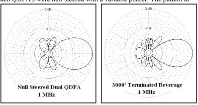
beverage. The 1 MHz NSDQDFA pattern above also gets progressively better than the beverage, especially if appropriate size flag elements are used in place of the delta flag elements. Furthermore, it is difficult to find a coastal site where you can put up a 3000' beverage pointed in the direction which you want to listen. A null steered dual QDFA array requires less than 800 feet of linear space.
